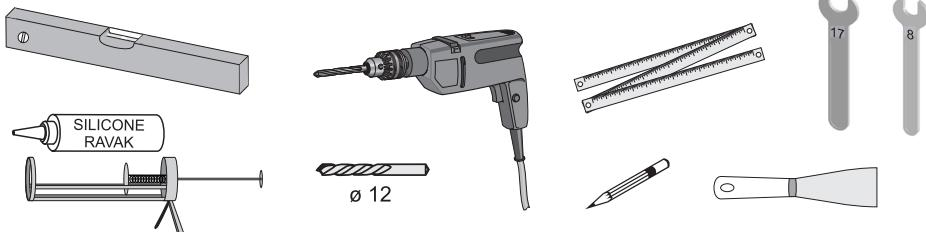
In order to secure the correct functioning, the product may be fitted only to solid walls of Bathrooms made of full bricks or concrete for which the enclosed wall plugs with screws are designed. When installing on the specific materials of the walls (porous concrete, hollow bricks or plasterboard) it is necessary to reinforce the place where the washbasin is positioned, by the structure with the sufficient load carrying capacity and use the corresponding wall plugs and screws.
